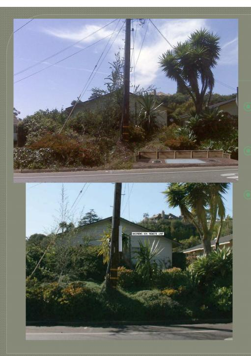
Vault requires 4' h x 14' l retaining wall Shrub removal required
