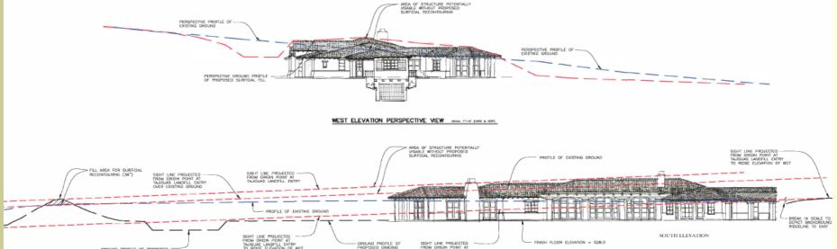
SIGHT LINE PROJECTED -----FROM CIRIGIN POINT AT TAJIGUAS LANDFILL ENTRY TO REDGE ELEVATION OF 807 OROUND PROFILE OF PROPOSED GRADING GROUND PROFILE OF PROPOSED GRADING FOR DRIVEWAY RAMP FOR UNDER-STRUCTURE PARKING SIGHT LINE SECTION 10410 (\*\*\*\*\*\*\* (\*042 & \*874)
