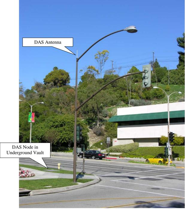
Figure 3: NextG Node Installed In An Underground Vault in Rolling Hills Estates, California.
