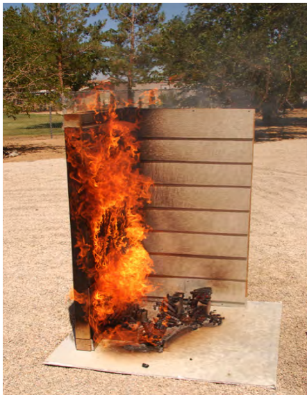
Vertical flame spread on the combustible siding product on the left-hand side of the corner section. The siding material on the right-hand side was a noncombustible product. A burning wood crib was the initial exposure for both wall sections. Source: firecenter.berkeley.edu/bwmg/siding-2.html
