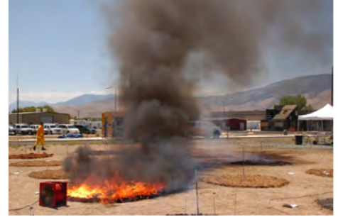
Burning rubber mulch during an experiment that evaluated various combustible mulch products. Source: Stephen L. Quarles
