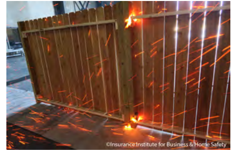
Ignition from ember accumulation most easily occurred at the intersection of the vertical planks and the horizontal lumber.
