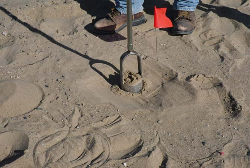
Collecting top auger sample of this hole.
