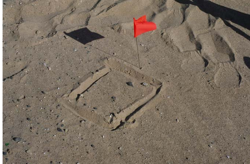
Approximate square foot for surface sample (~2" depth)
