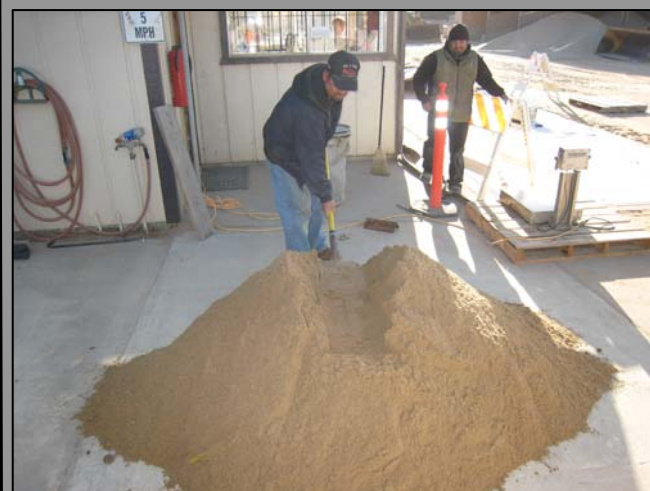
Cone and quarter sample size reduction
