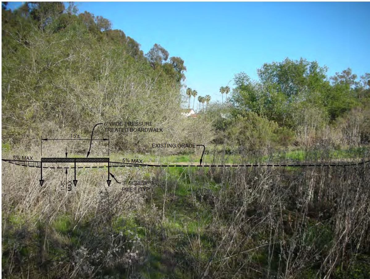
Devereux Creek: The proposed trail reconfiguration would include a boardwalk bridge across Devereux Creek, which would be constructed with screw piles similar to Drainage A. The crossing would be approximately eight feet wide and 60 feet in length.
