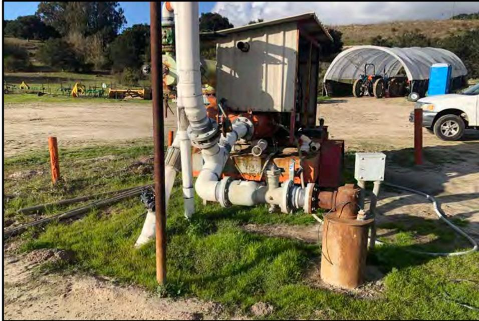
*Photo 1. The 10-inch-diameter PVC-cased cannabis irrigation well, with 16-inch-diameter steel sleeve shown above grade.*
