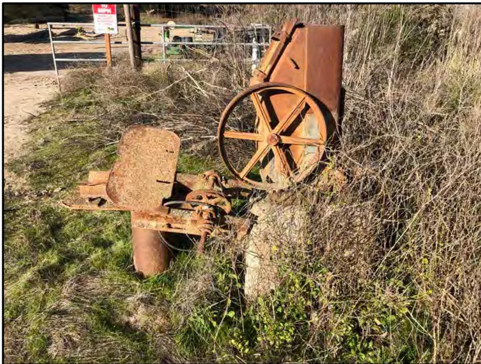
*Photo 2. The 6-inch-diameter mild steel-cased inactive windmill well encased in concrete pedestal.*
