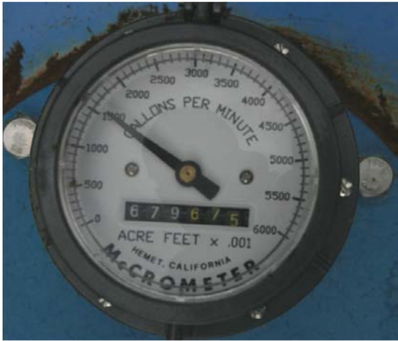
Figure 3: Example Flow Meter Display (Totalizer reads 679.675 acre-feet)
