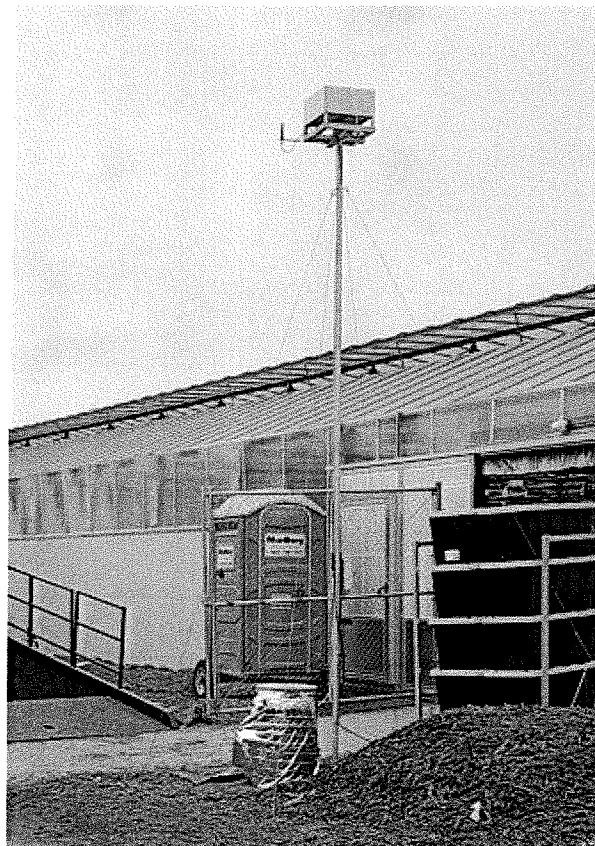
Figure 3. Sample tubing was run up the pole to collect air at roof vent elevation
