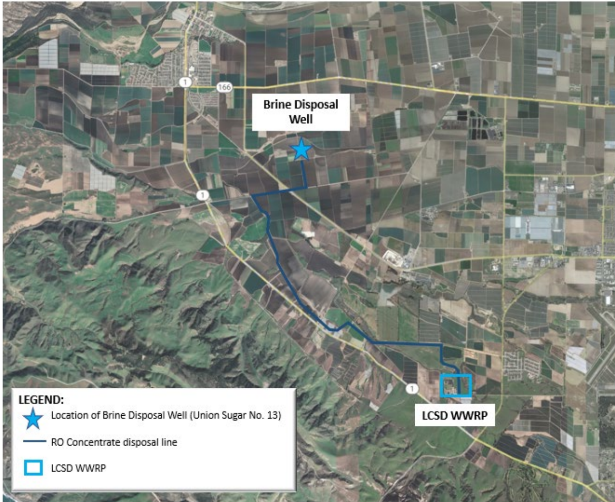
Figure 3.6 RO Concentrate Brine Disposal Line and Disposal Well
