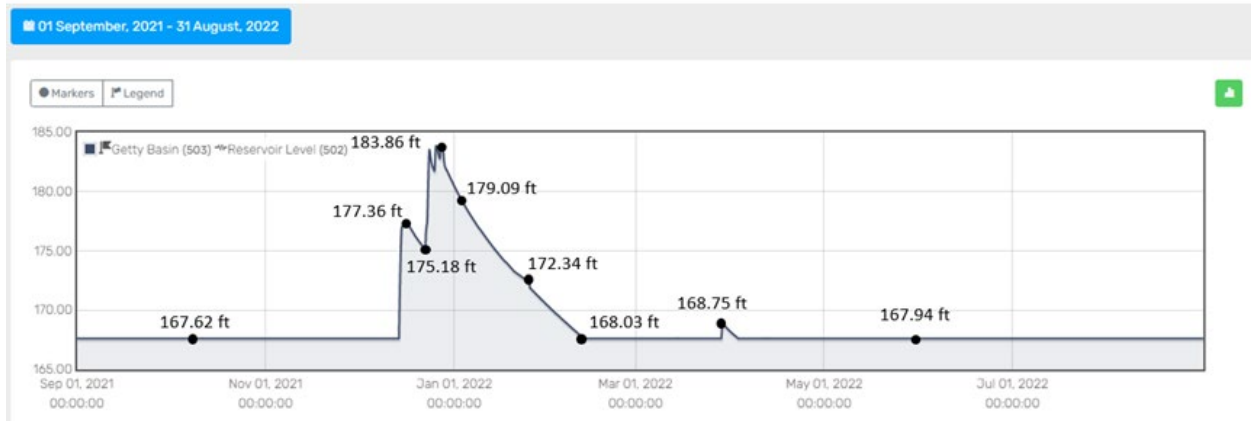
Figure E.3 Getty Basin Reservoir Level – Wet Year (2021-2022)
