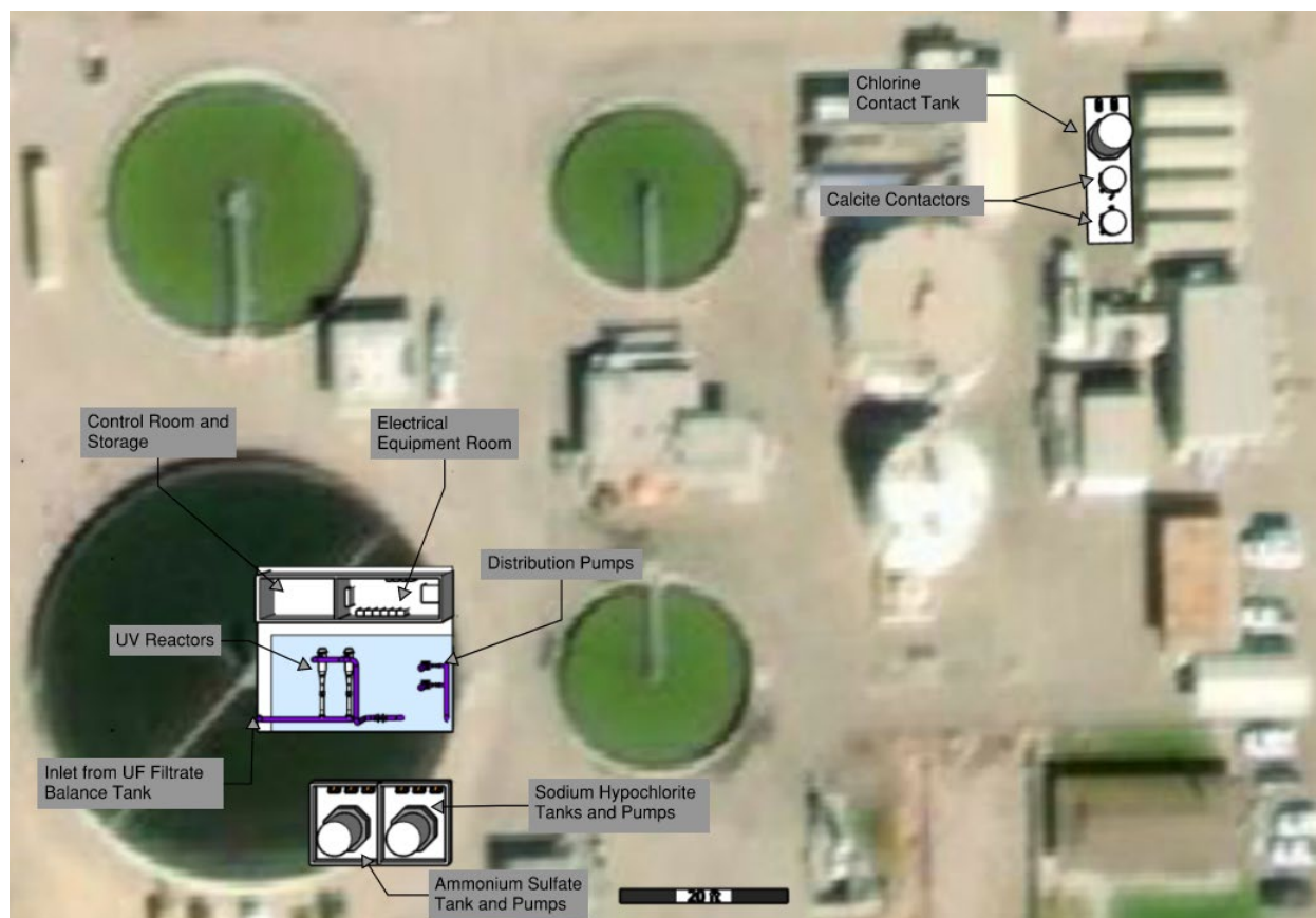
Figure 5.3 Fast Track Site Layout – new UV system and upgrades to existing UV system (Plan View)
