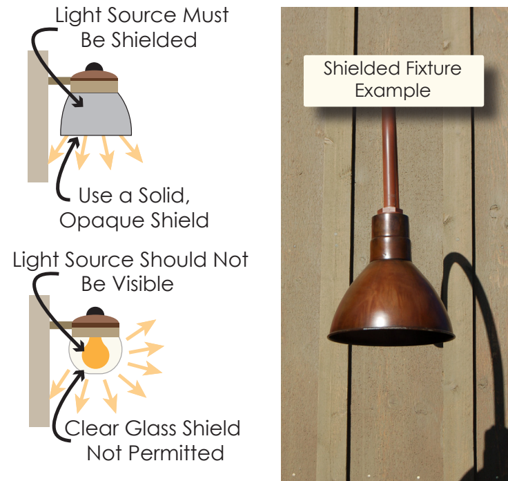
Figure 6.10 – Shielded Lights Versus Non-Shielded Lights
