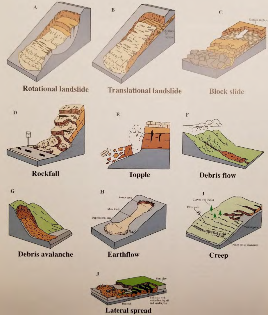
Figure 3. These schematics illustrate the major types of landslide movement that are described in the previous pages. For additional information on these processes and where to find photos, please see "Where to Go For More Information" at the end of this fact sheet.
