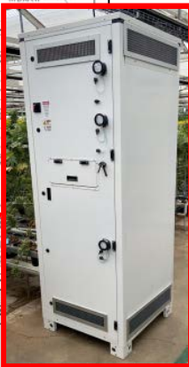
Typical-Regenerative Carbon Scrubber System
