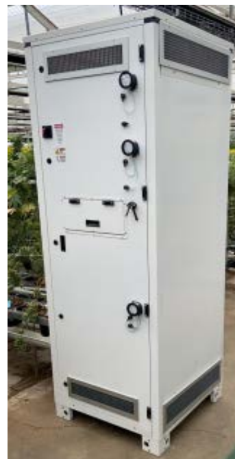
Figure 5- Prototype Regenerative Carbon Scrubber System
