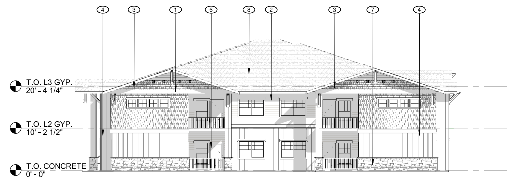
3 WEST ELEVATION - BLDG. TYPE B 3/32" = 1'-0"
