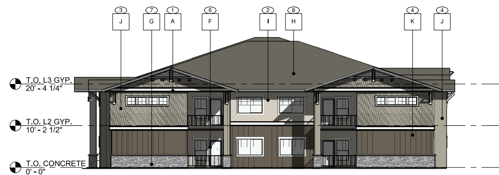
③ WEST ELEVATION - BLDG. TYPE B 3/32" = 1'-0"
