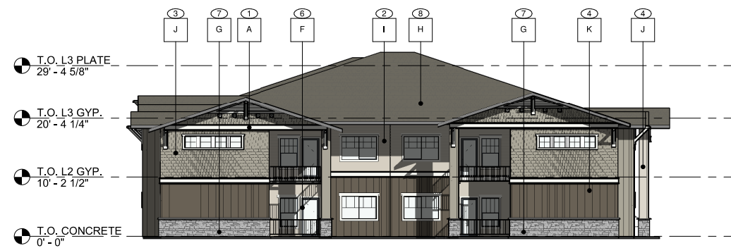
② EAST ELEVATION - BLDG. TYPE B1 3/32" = 1'-0"
