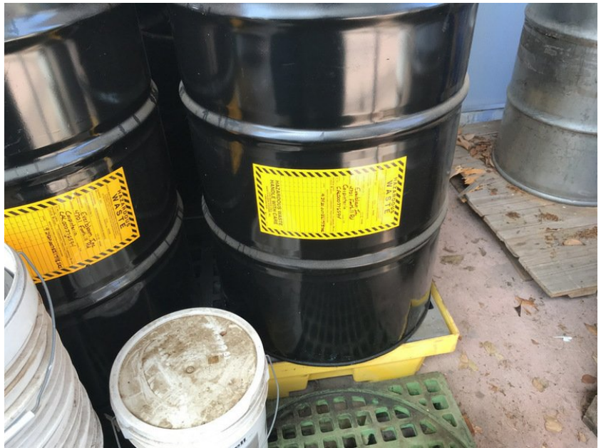
Remove waste oil. Relocate to an area away from the runoff pond.
