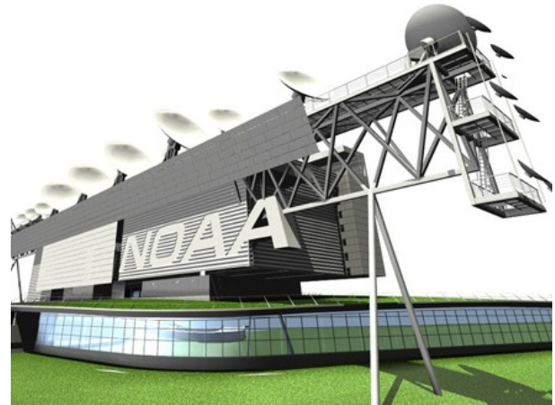
Figure 2-14. Green Roof of National Oceanic and Atmospheric Administration, Suitland, Maryland. Vegetated, or green, roofs can contribute to the reduction of heat islands (LEED Sustainable Site Credit 7.2: Heat Island Reduction – Roof) as well as the reduction of stormwater runoff (LEED Sustainable Site Credit 6.1: Stormwater Management – Rate and Quantity) Architect: Morphosis (Rendering: Morphosis)
