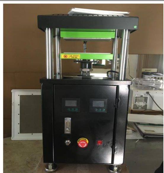
Our team has met with cannabis manufacturers to review techniques such as this rosin press which uses heated plates to press cannabis at 300 to 600 pounds per square inch to convert trimmings into rosin, a product with high THC content.
