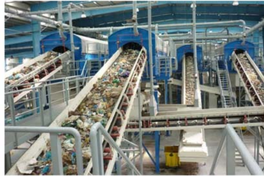
Larnaca, Cyprus Mixed MSW Dirty MRF similar to BYS Warsaw, Poland & proposed design for Santa Barbara (comparable waste composition) Constructed in 2009
