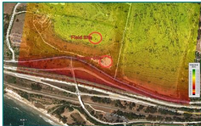
Figure 1: Sound Level Contours near Lambert Road and U.S. Highway 101. Two proposed landing sites are shown, designated "Field Site" and "Corner Site"
