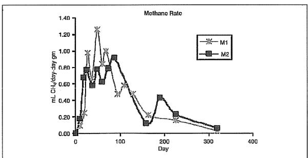
Fig. 1. Generation of methane in experimental apparatus simulating landfill bioreactions (M1 and M2 denote two different tests; [14]).
