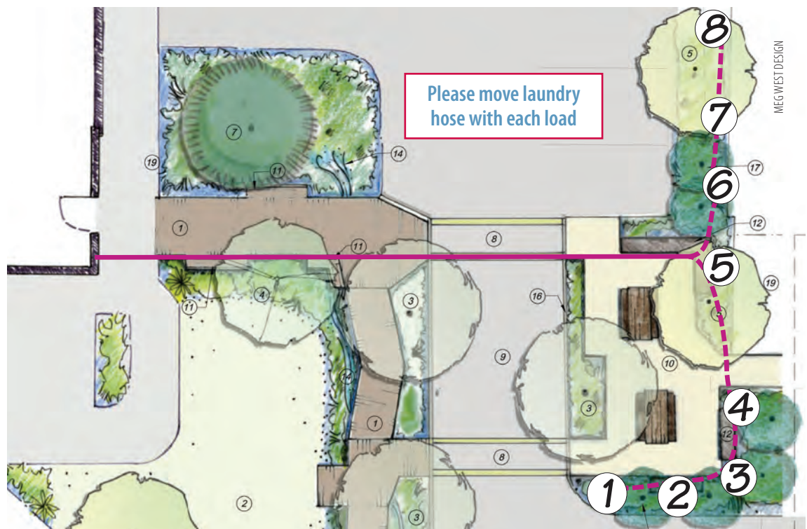
Sample map of outlet moving sequence to post by the washing machine. When you start a load, you move the hose to the next spot; from 1 to 2 to 3, etc.
