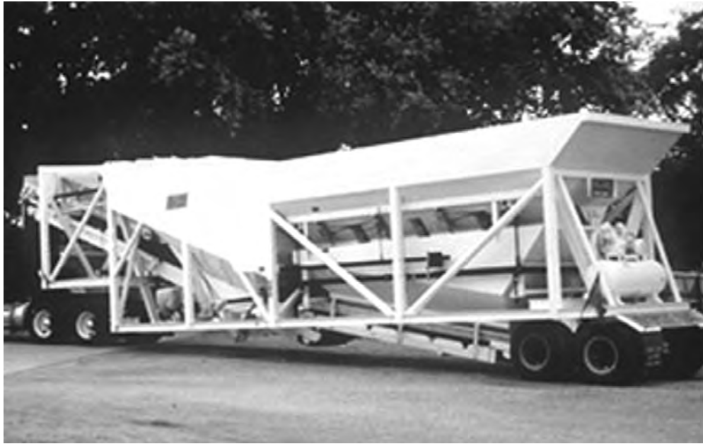
Batch Plant during Transport
