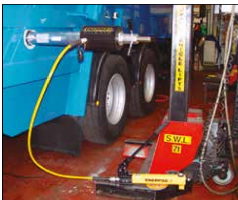
◀ An RACH-306 powered by a P-392 hand pump used to extract corroded carriage pins of refuse collection vehicles.
