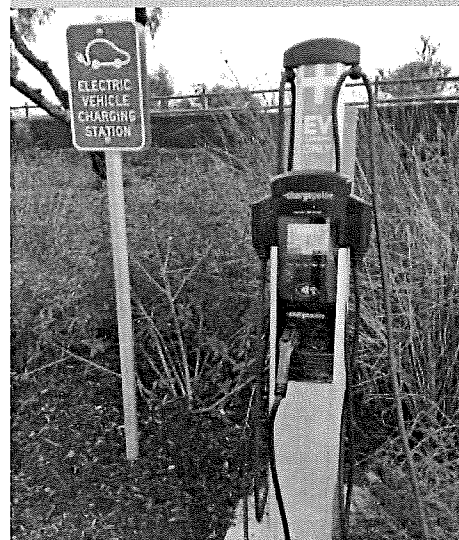
Electric vehicle charging stations like this will be tested by weights & measures officials
