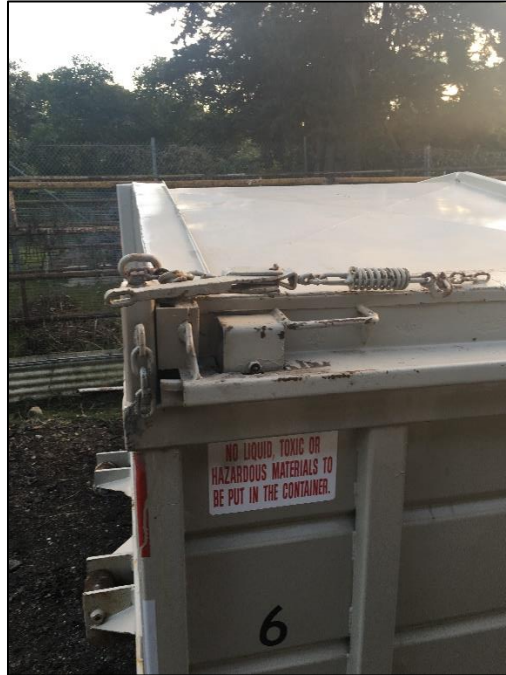
Figure 7. Locking Mechanism of Waste Bin Onsite.
