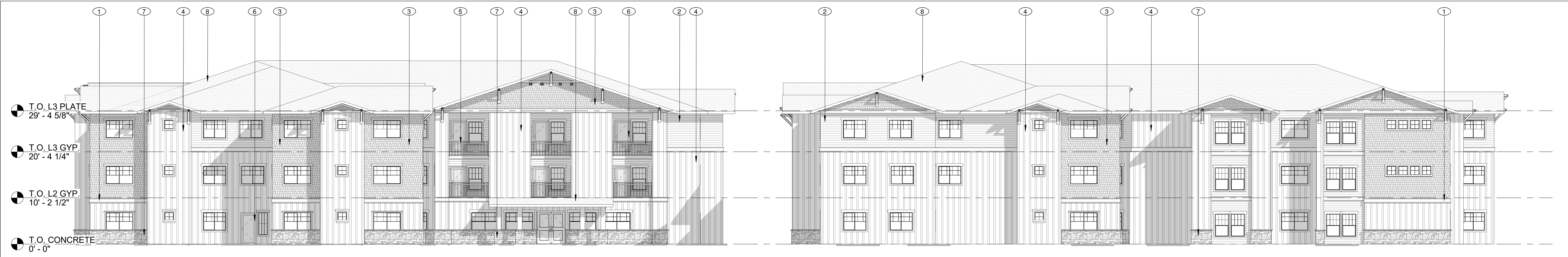
① EAST ELEVATION - BLDG. TYPE A 3/32" = 1'-0"
