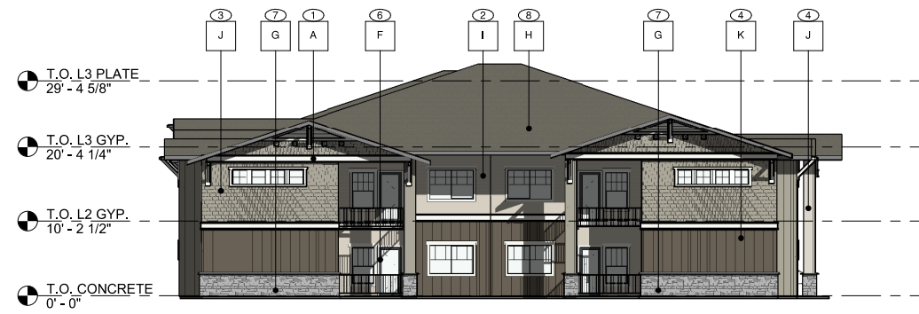
② EAST ELEVATION - BLDG. TYPE B1 3/32" = 1'-0"
