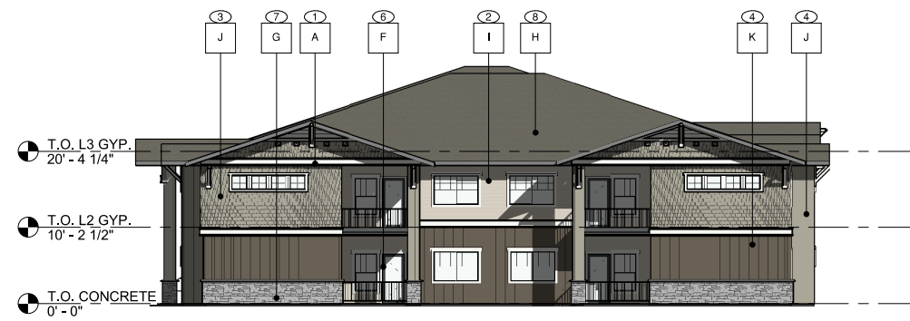
③ WEST ELEVATION - BLDG. TYPE B 3/32" = 1'-0"
