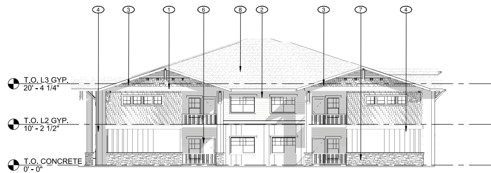
③ WEST ELEVATION - BLDG. TYPE B 3/32" = 1'-0"
