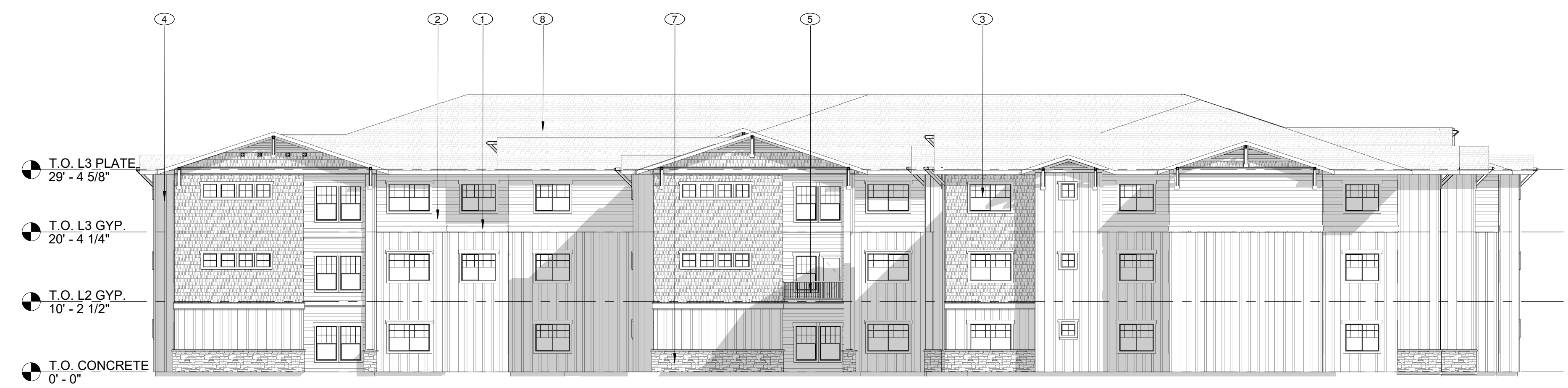
③ NORTH ELEVATION - BLDG. TYPE A 3/32" = 1'-0"
