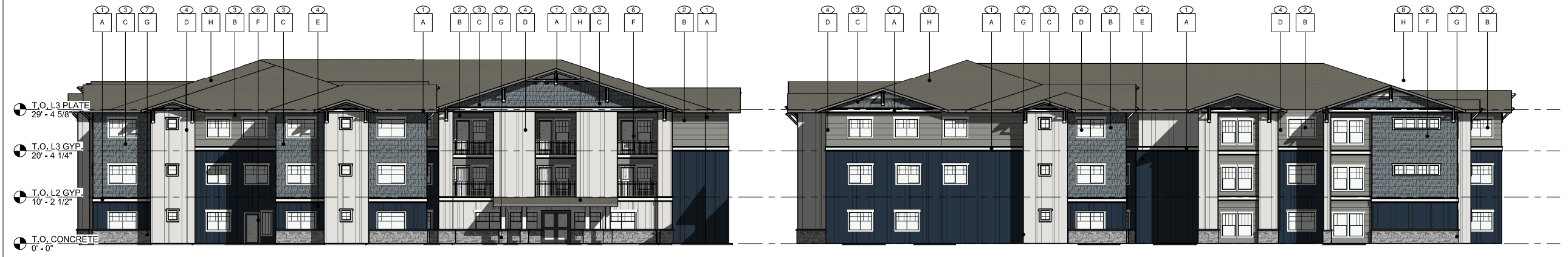
1 EAST ELEVATION - BLDG. TYPE A Copy 1 3/32" = 1'-0"
