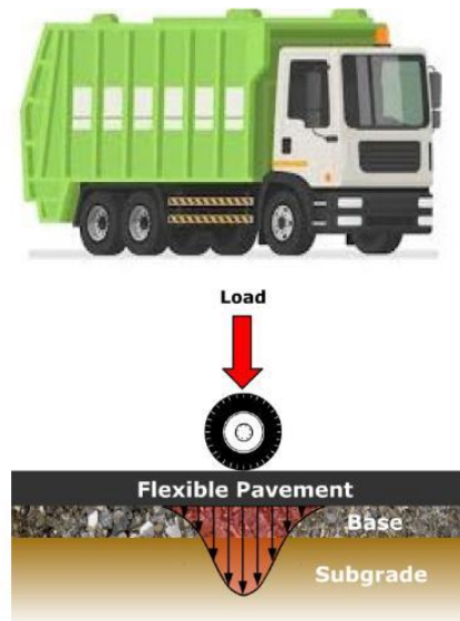
Figure 1. Vehicle Impact on Pavement
