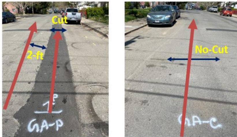
Figure 4. Falling Weight Deflectometer (FWD) Testing Layout
