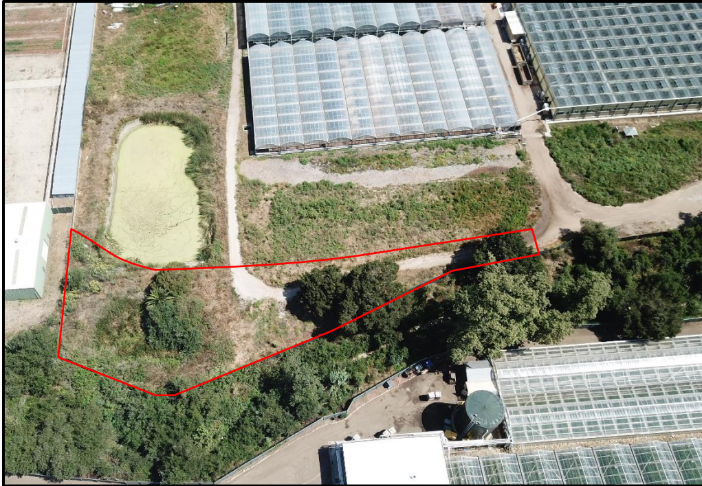
Photo 9: Drone photograph of the southwest corner of Project Site, bioswale, detention basin, and approximate Riparian Restoration Area (red outline). Photo taken July 7, 2020.
