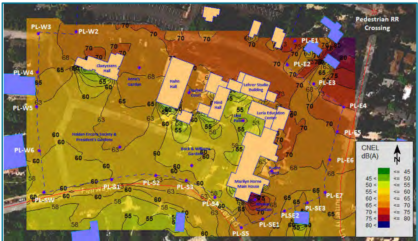
Figure 8: CNEL Noise Contours for 3-Hour Event at Kinnear Fountain with Source Power Level of 105 dBA
