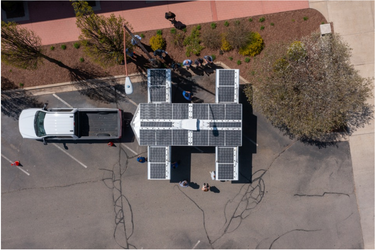
Sesame Solar Nanogrid Mobile Power Solution – Full Deployed Solar Array
