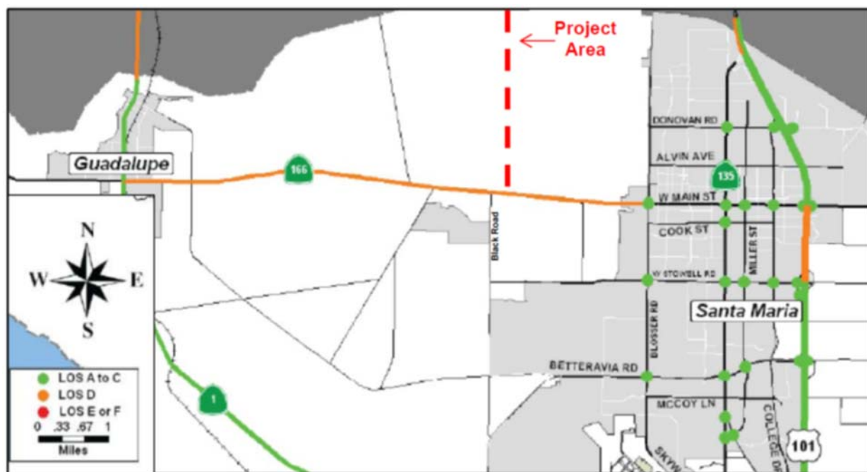
Figure 5.15-1. Santa Barbara County, Congestion Management Plan Map Showing LOS levels in the Project Area
