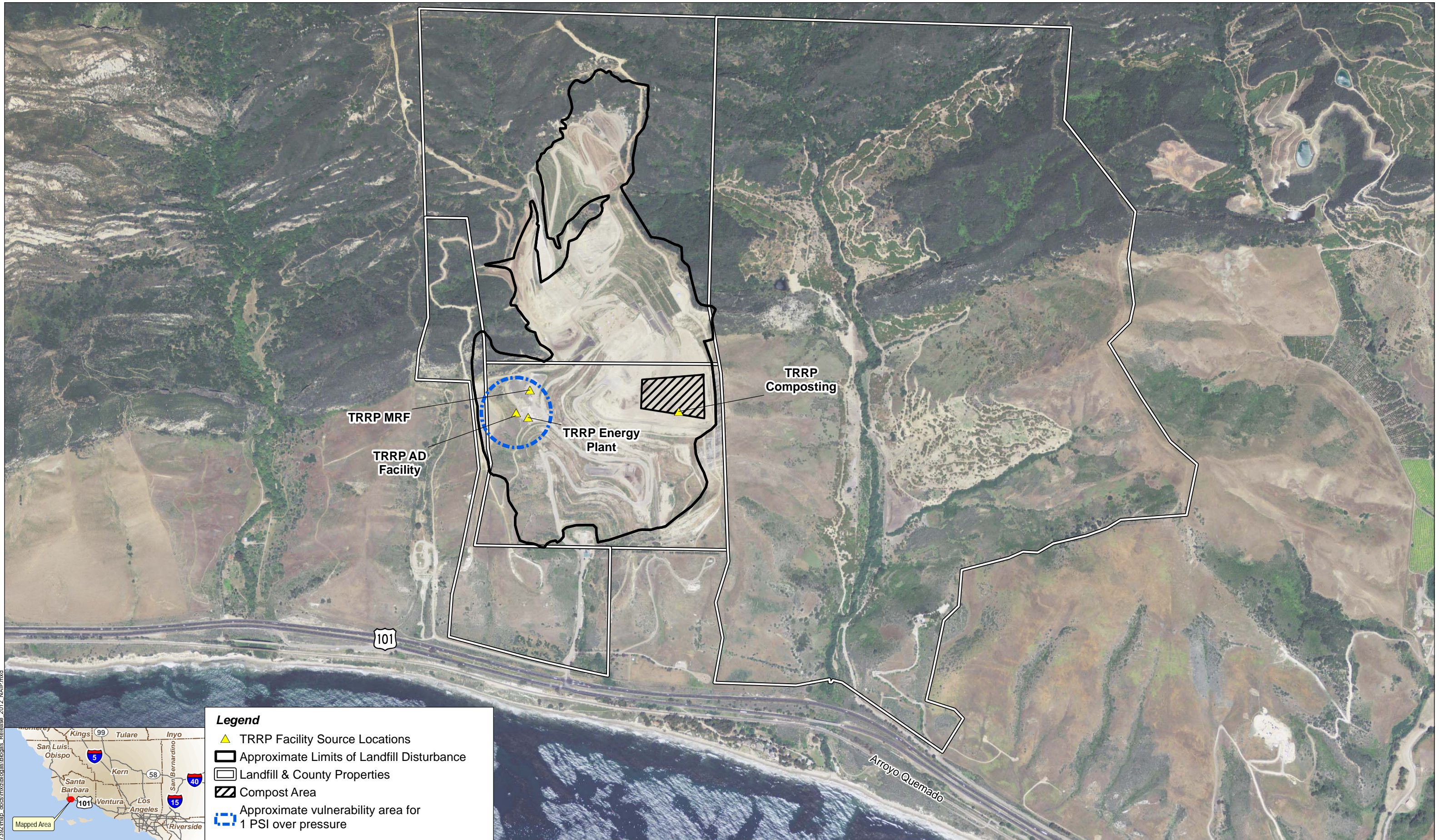
Figure 1. Tajiguas Resource Recovery Project Vulnerability Area for Biogas Release Resulting in Explosion
