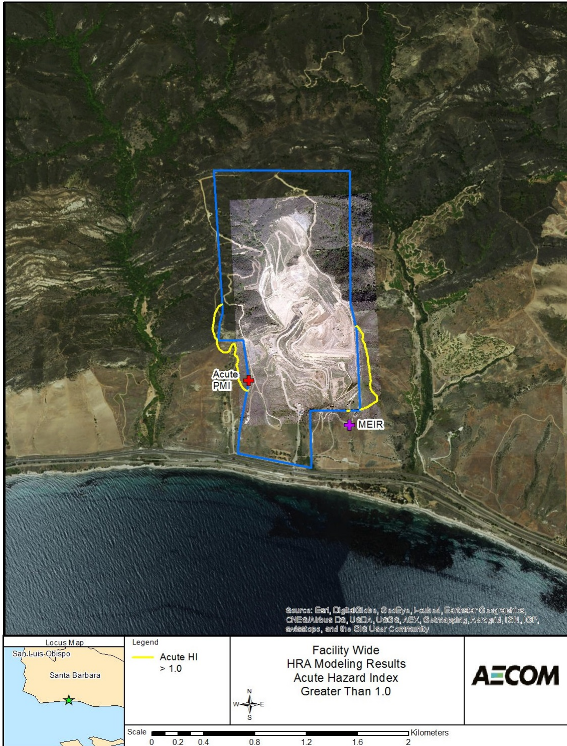
Figure 6-2 Acute Hazard Index Isopleth Greater than 1.0 for Future Operations at Tajiguas Landfill with TRRP and CSSR
