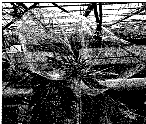
Figure 3. Example of leaf enclosure system used to develop emission factors.
