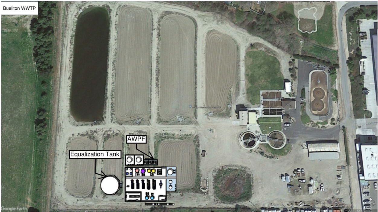
Figure 4.7 IPR AWPf Zoom-Out Site Plan of Buellton and Solvang Combination for 0.78-mgd Production
