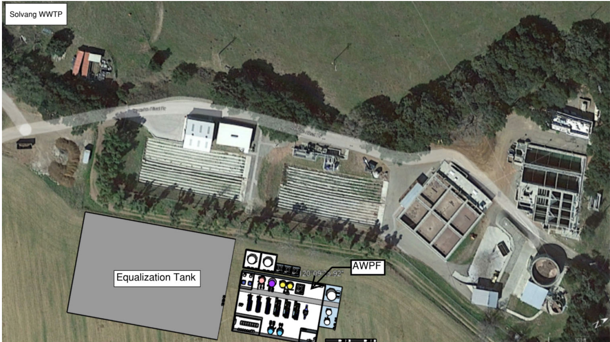
Figure 4.6 Solvang IPR AWPf Zoom-Out Site Plan for 0.76-mgd Production
