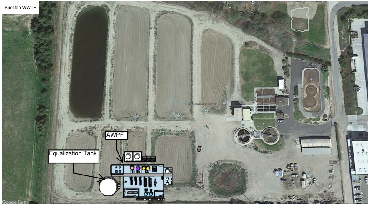
Figure 4.5 Buellton IPR AWPF Zoom-Out Site Plan for 0.33-mgd Production
