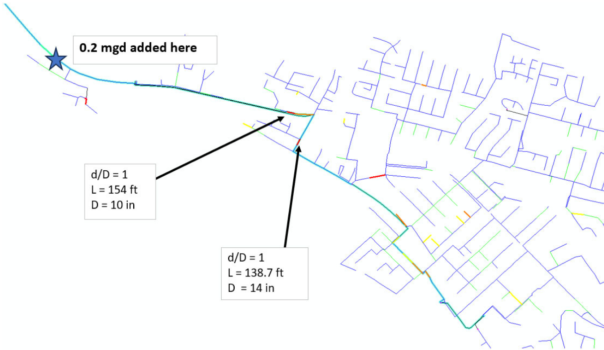
Figure 5.16 Modeled Gravity Mains Exceeding d/D = 0.92 (0.2 mgd Flow Scenario)
