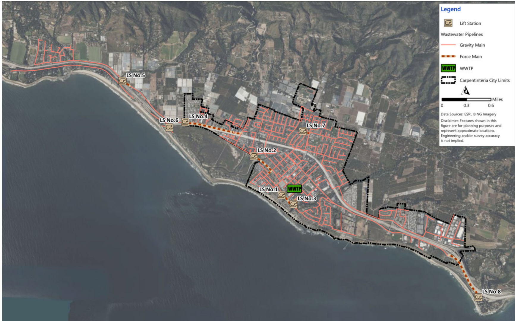
Figure 5.14 CSD Wastewater Collection System
