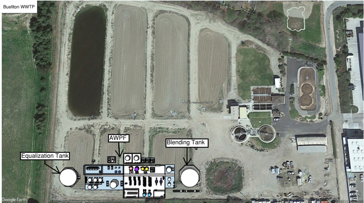
Figure 4.10 Buellton DPR AWPf Zoom-Out Site Plan of Buellton and Solvang Combination for 0.73-mgd Production
