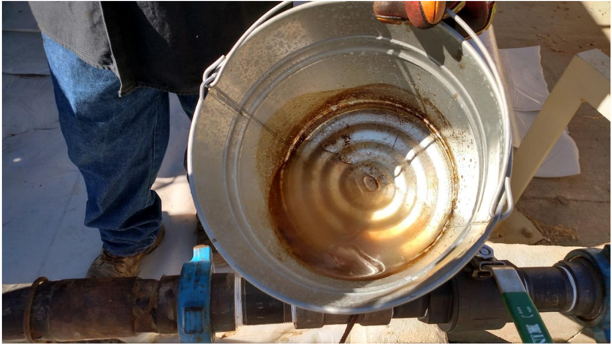
Photo 1: Sample of water that was recovered from the Tautrim pig receiver
