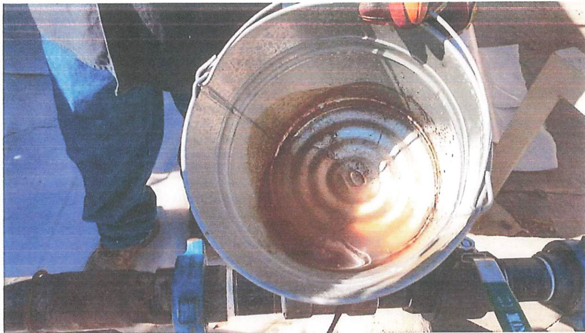
Photo 1: Sample of water that was recovered from the Tautrim pig receiver
