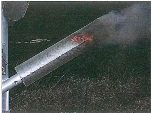
Figure 2.4 Flare burning inside spark arrestor
