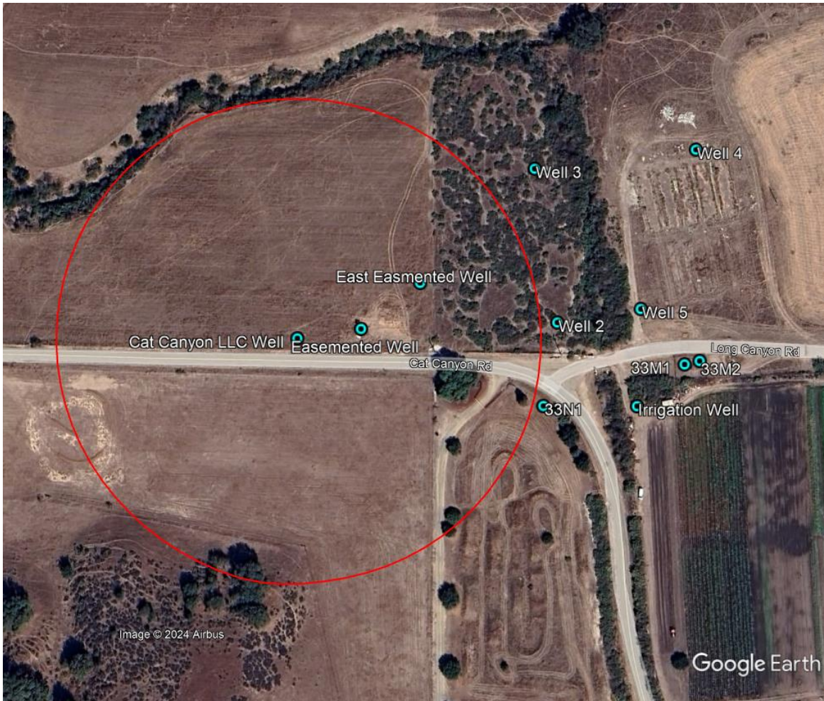
Figure 3. Cat Canyon LLC production well indicating 400-foot radius which represents modeled limit of 0.1-ft water level drawdown with 14 hours of pumping at 10 gpm; creek and off-property wells are outside of this radius.
