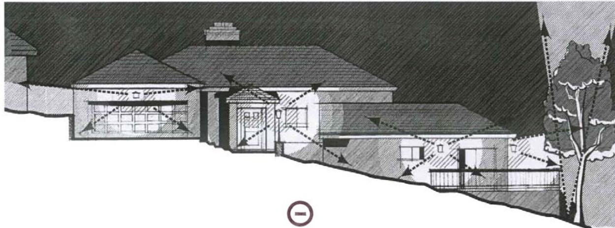
Unshielded light fixtures resulting in light escaping onto neighboring property and into the night sky
