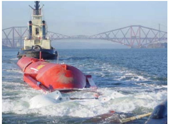
Fig. 7-1. The Pelamis attenuator, developed by Ocean Power Delivery of Scotland.
