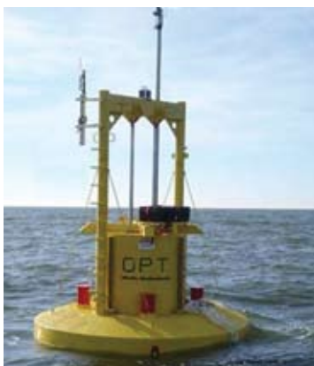
Fig. 7-2. Ocean Power Technologies PowerBuoy, as seen from above water.
