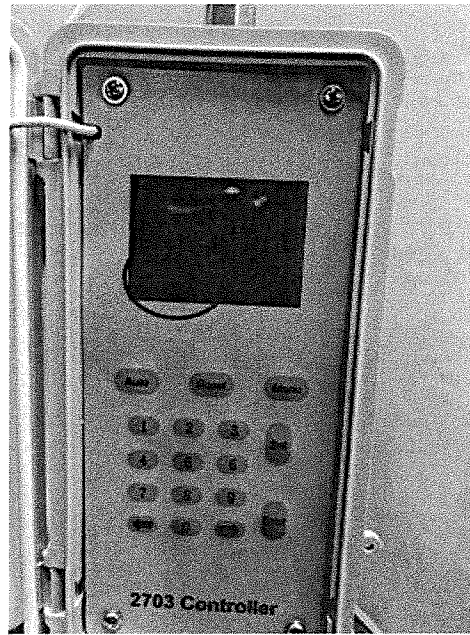
Figure 15: Manually setting the flow rate on the Nutech 2703 controller.
