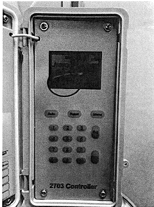
Figure 16: Manually setting the stop time and flow rate.
