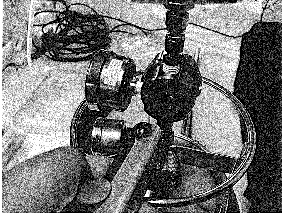
Figure 7. Using a 3mm hex key wrench to adjust piston gap screw.
