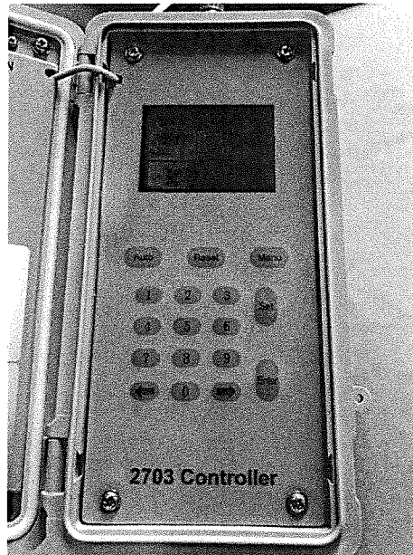
Figure 18: Nutech 2703 controller has started a scheduled sampling event.
