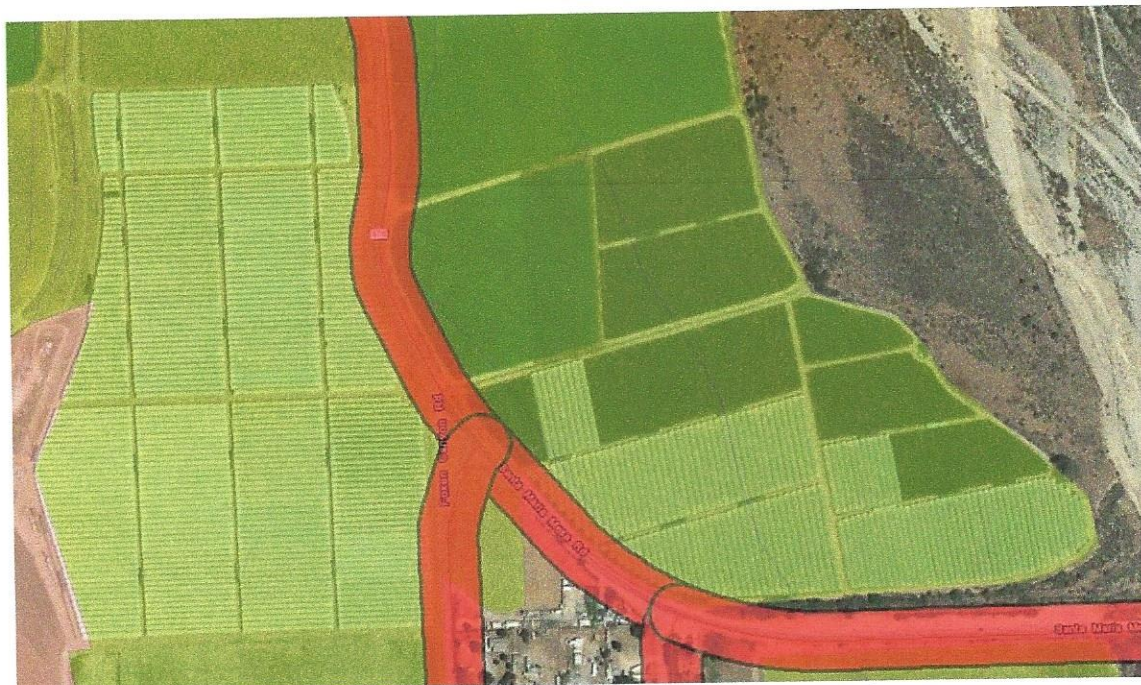
Example of impacts of 75-foot road setback limiting height to 12-foot hoops (MM-VIS-1)
