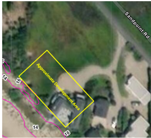
Figure 2 . Air Photo view of the site with water surface elevation contours (courtesy of FEMA) 1
