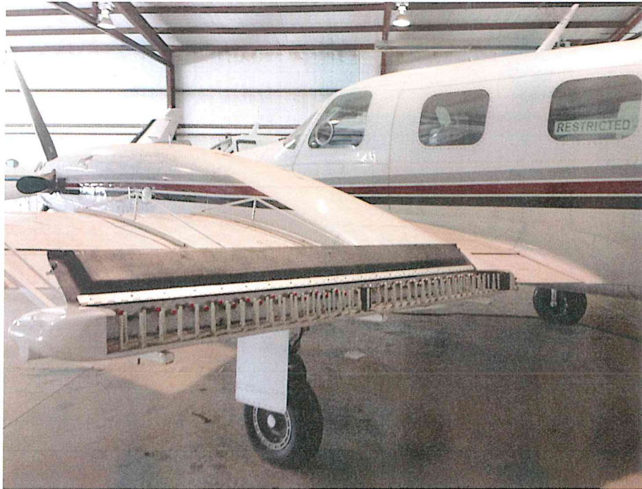
Figure 2.7 Cheyenne II burn in place flare rack
