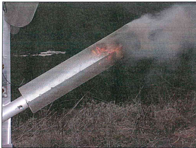
Figure 2.4 Flare burning inside spark arrester
