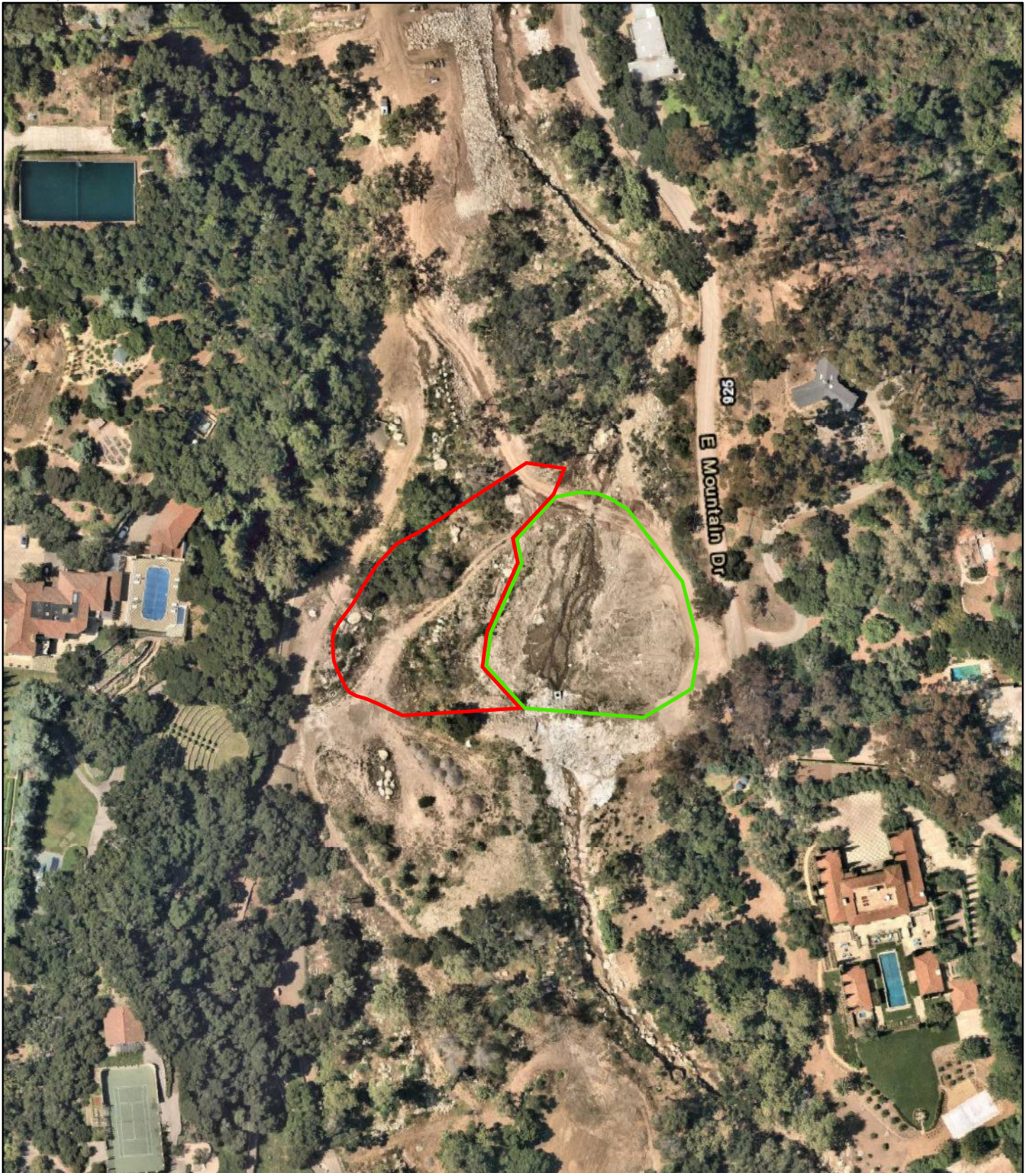
FIGURE 2 Existing Cold Springs Debris Basin and Expansion Area Overview Cold Springs Debris Basin Expansion Santa Barbara County, CA.
