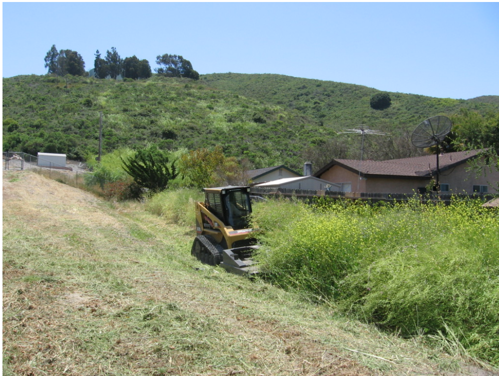
Low ground pressure rubber tracked mower to reduce herbicide use
