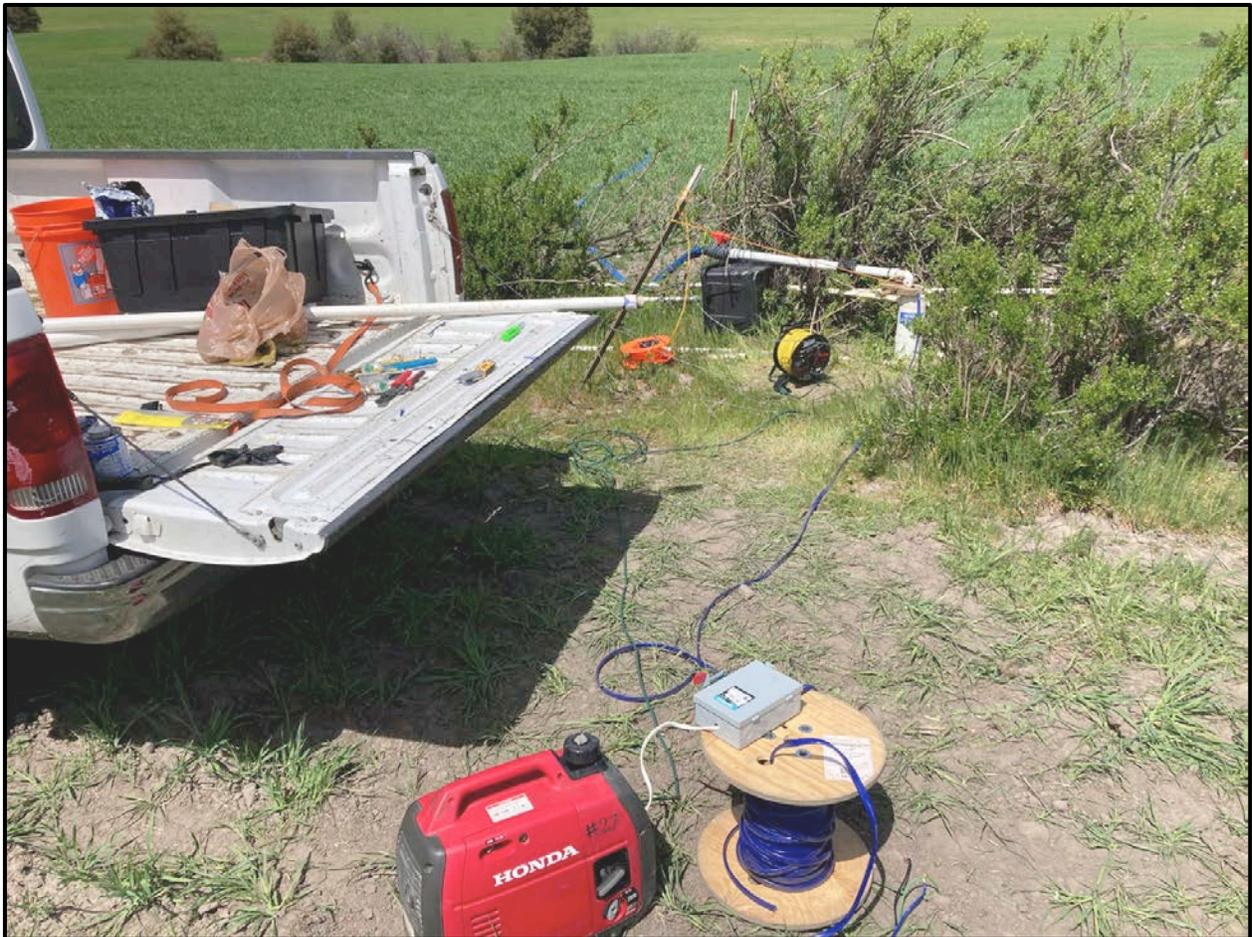
***Photograph 1. Source yield testing the western 5-inch-diameter PVC well at APN 101-070-069 (KG, 14-April-2021).***
