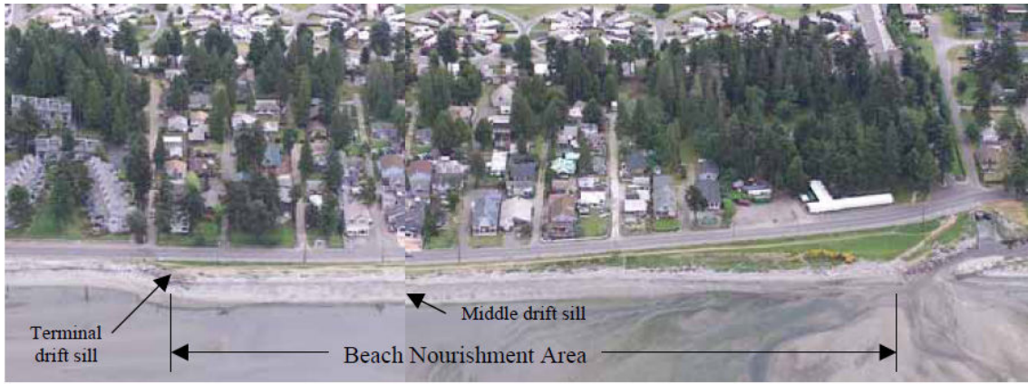
Figure 1. Oblique aerial photo mosaic of the study site, located immediately left (north) of the mouth of Terrill Creek (at right). Photos taken May 24, 2001 for WA Dept. of Ecology.
