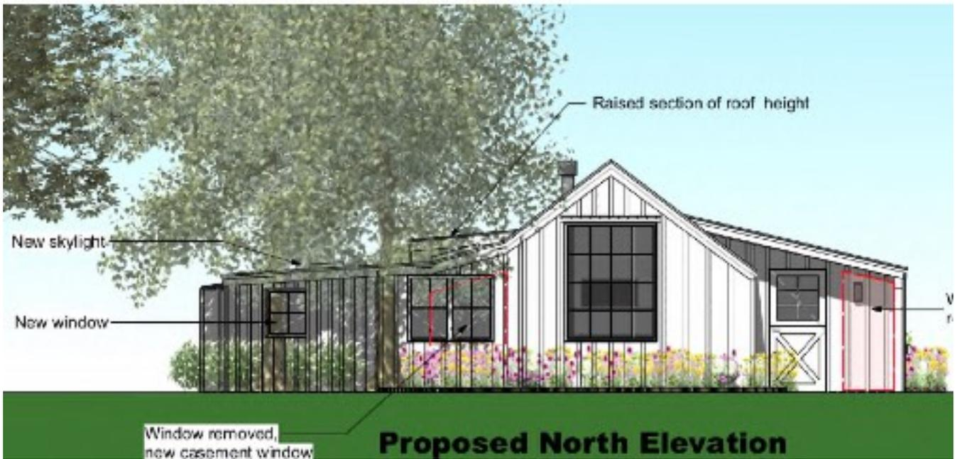
Figure 22, Proposed north elevation
