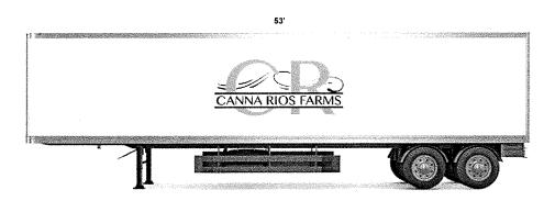
53 ft semi-trailers have a capacity of 3,489 cu ft (cubic feet) and weigh 13,500 lbs.
